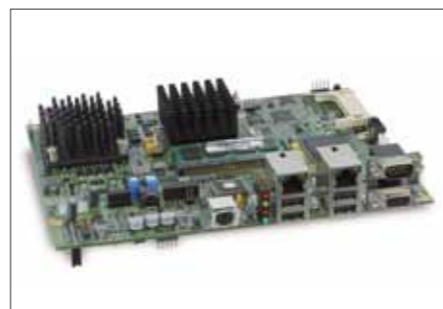
Image 1: Industrial fieldbuses add-on cards Image 2: PCI slot for expansion cards Image 3: Intel Celeron M and Pentium M processors up to 2GHz
