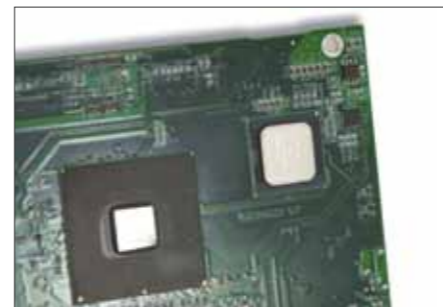
Image 1: Closed enclosure Image 2: 2 MiniPCI expansion slots Image 3: Intel ATOM processors
