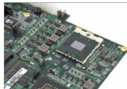
Image 1: Keyboardless version Image 2: 4 PCI/PCIe slots on H4 version Image 3: Intel Core 2 Duo microprocessors and 965GME chipset
